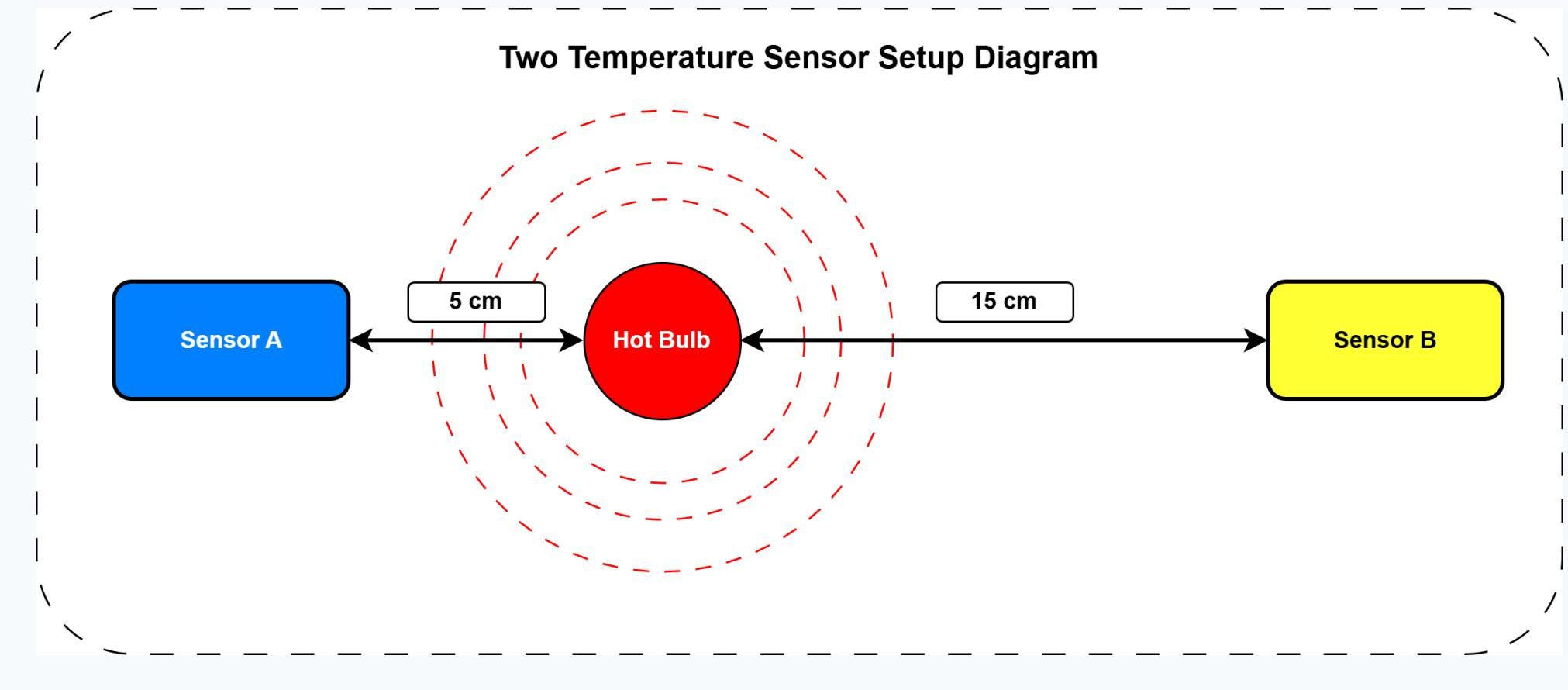
Schematic: Sensor A (close, high noise) and Sensor B (far, low noise).
